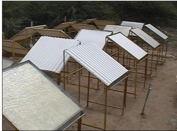
Figure 3. Different Types of Condenser Surfaces Investigated (Sharan, 2011)
